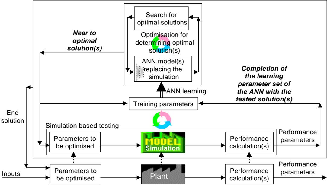
**Fig. 3.** Concept of the hybrid, AI-, ML- and simulation-supported optimisation of production plants
