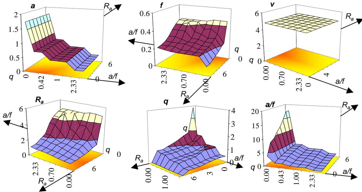
**Fig. 2.** Parameters resulted by the threefold optimisation of the plate turning operation
